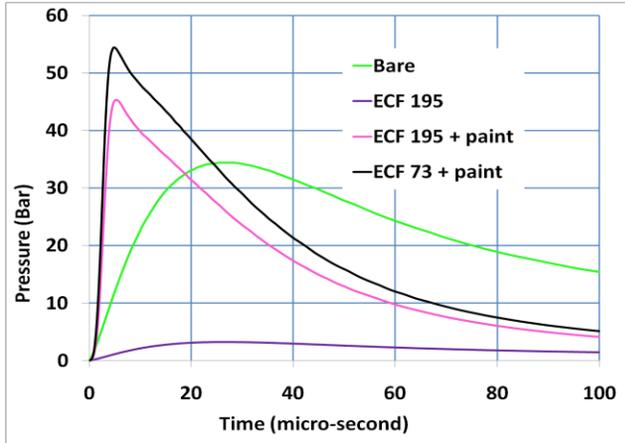
**Figure 4: Pressure at the surface of the composite material, as a function of time, obtained with the simple surface explosion model.**
