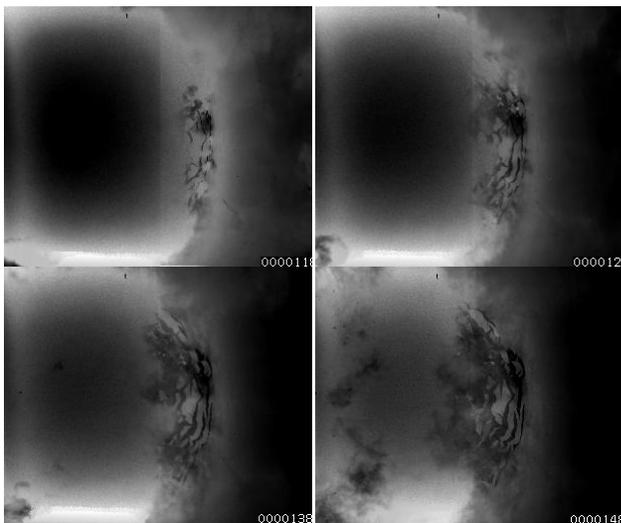
**Figure 2: Pictures of the strike in its extinction phase. Ordered from top left to bottom right, the pictures are separated by 10  $\mu$ s. The first one corresponds to nearly 78  $\mu$ s after initiation.**
