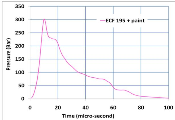
**Figure 6: Pressure on the surface as a function of time for  $r=6$  mm (arc root radius), obtained with ABAQUS.**
