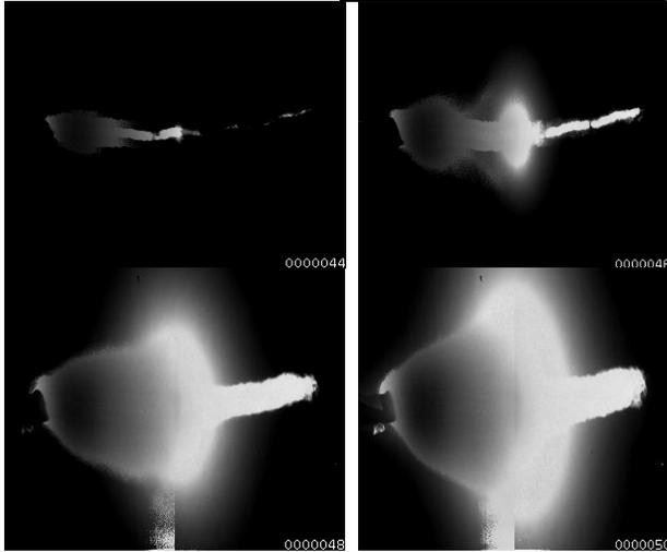
**Figure 1: Pictures of the strike in its initiation phase. Ordered from top left to bottom right, the pictures are separated by 2  $\mu$ s. The arc was initiated less than 2  $\mu$ s before the first picture. Right part of the picture corresponds to the reflected image of the arc on the sample. The electrode is on the left.**
