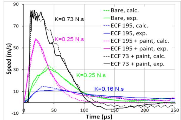
**Figure 3: Speed of the sample at the strike point as a function of time. Different samples are considered. Continuous line : experimental result. Dashed line : model. K is the impulse (in N.s) corresponding to the surface pressure integrated over area and time.**
