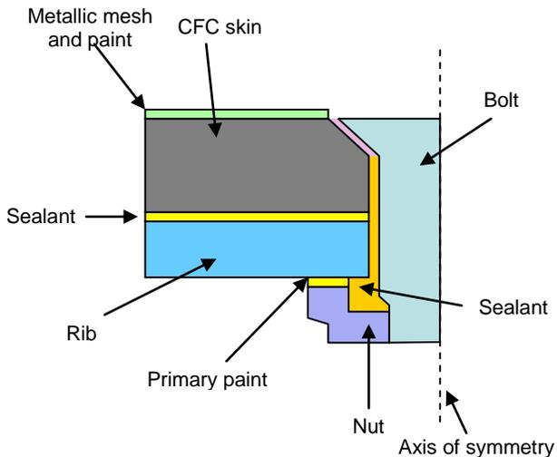
Figure 1. Junction at the fastener scale.
