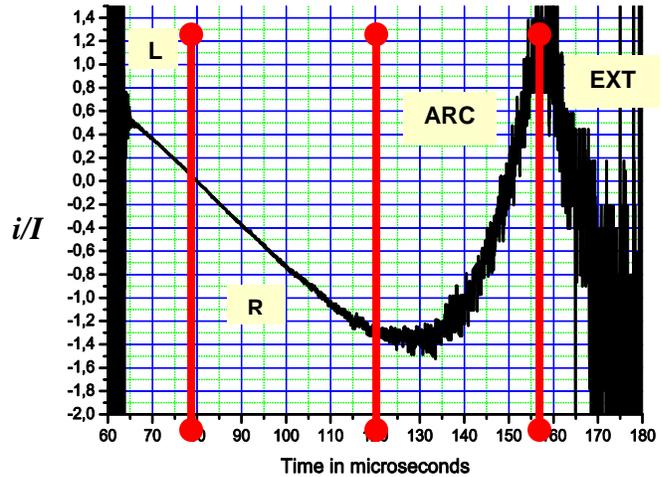
Figure 4. Time dependence of the relative differential current  $i/I$ . The vertical lines define four time intervals. The ones labeled “L”, “R” and “ARC” correspond to intervals where one of the three generators (eq. (2)) dominates the others (#2 in “L”; #1 in “R” and #3 in “ARC”). In region “EXT”, all generators extinguish and the currents become small and noisy.
