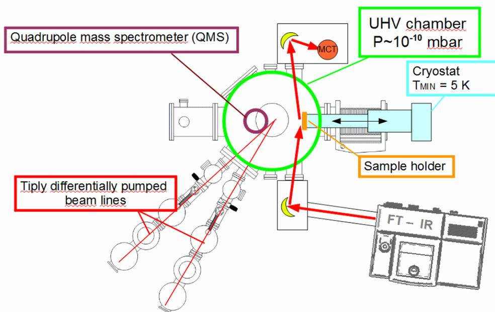
FORMOLISM consists of a UHV chamber, in which an HOPG temperature-controlled in the 6 - 400K range can be located. The sample will be heated up-to 1000 C in a separate preparation chamber and glued to a gold mirror.
