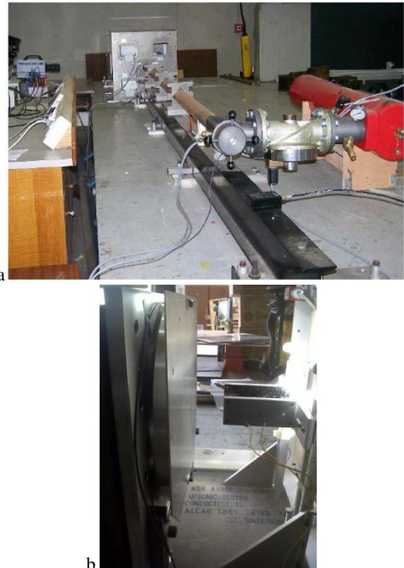
Figure 3: Gas gun apparatus: a): complete set-up with the pressure vessel; b): the metallic boundary ring on which is fixed the target square plate.
