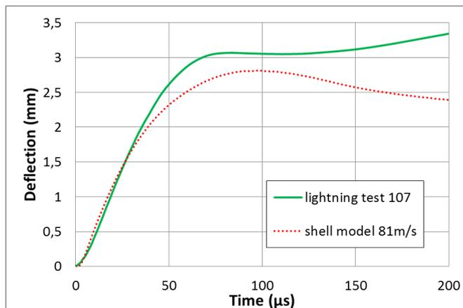
Figure 2: Comparison of rear face deflections between lightning strike (plain line) and numerical simulation with a steel projectile (dotted line).
