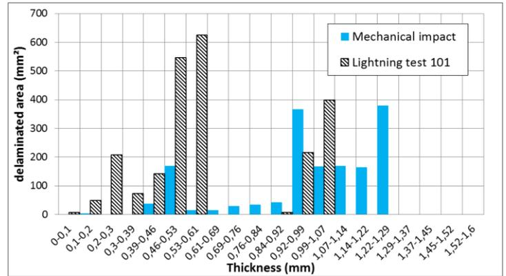
Figure 8: Histograms of the delamination as a function of position in the thickness (as defined in fig. 6) of the material, for # 101 (top) and # 107 (bottom) samples.
