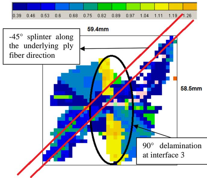
Figure 7: ultrasonic scans for lightning strike (top) and associated mechanical impact (bottom) at 75m/s for sample 101 at interface between plies 3 (-45°) and 4 (90°).
