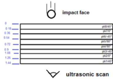
Figure 6: Two scales for ultrasonic testing method: left the thickness, right the fibre orientation
