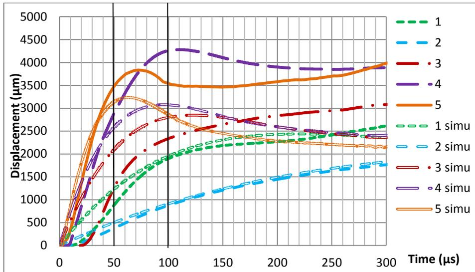
Fig. 3: Deflection vs time for the impact computations (full lines) and lightning strike tests (dotted lines).
