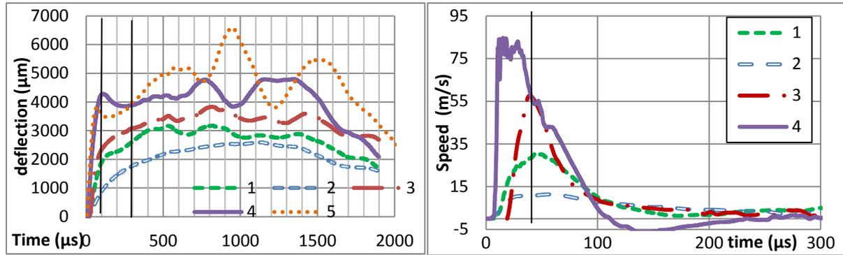
Fig. 2: (a) Deflection as a function of time of the central point at the rear side of the sample subjected to a D waveform lightning strike. (b) Velocities as a function of time for the first 4 samples.
