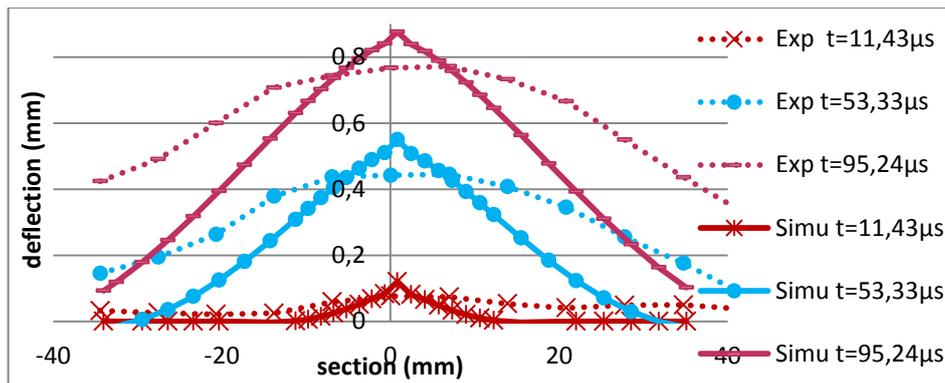
**Fig. 4:** Deflection of the central portion of the samples vs time. Full lines: impact simulations; dotted lines: lightning strike tests. Top: CFRP1, sample 2; bottom: CFRP2, sample 5.
